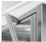
Replaceable gaskets with high level of insulation Triple chamber geometry with innovative D7 compound, which produces 35% higher insulation efficiency than traditional models.
